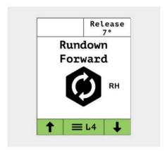
With Speed Switch in Rundown select Loosen on the direction switch to run off nuts.
